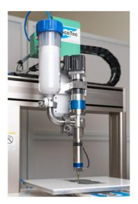
The vipro-PUMP series are optimised dosing components and a modular construction provide numerous opportunities for adapting the dosing equipment even more effectively to the relevant application. For process reliability with precise dispensing results. The control unit can be easily integrated into fully automatic systems and meets all requirements of a modern dispensing process. The vipro-PUMP will be available in five different sizes (dosing volume of approx. 0.14 to 5.2 ml/rev)
