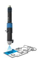
The preeflow eco-SPRAY enables volumetric precision dispensing based on the endless piston principle. The basis is a rotating, fully pressure-tight displacement system. It consists of a rotor and stator. The defined rotary movement of the rotor displaces the material volumetrically in the stator. This creates the flow. Controlled via the processor, a defined quantity is fed into the special low-flow spray chamber.
